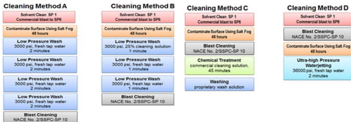
Figure 1: Diagram Showing Individual Steps Involved in the Contamination and Four Cleaning Methods
